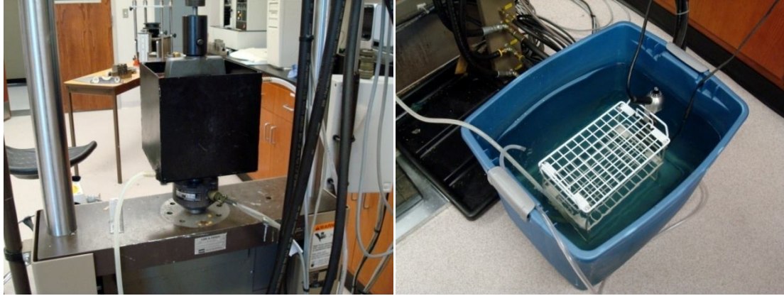
Figure 21: The water bath seen on the left circulates the water until the specialized chamber shown by the tubing connections on the photo on the right. The water is pumped in through the base of the chamber and returns to the reservoir through the top tubing.
