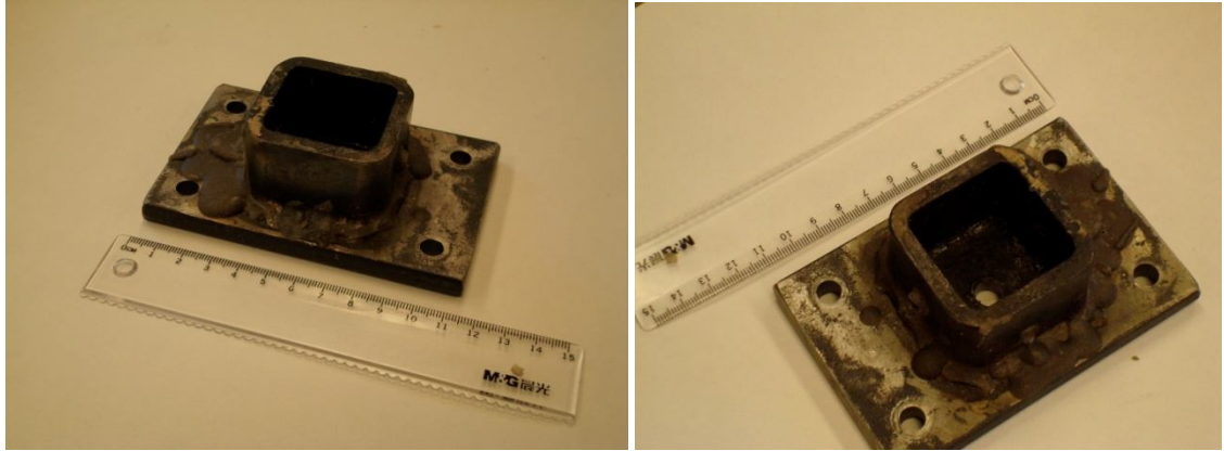
Figure 16: The specially designed pots in which the tibial section of the specimen was held in place. The pot also was able to be bolted down to the specialized water chamber as seen below in Figure 19.
