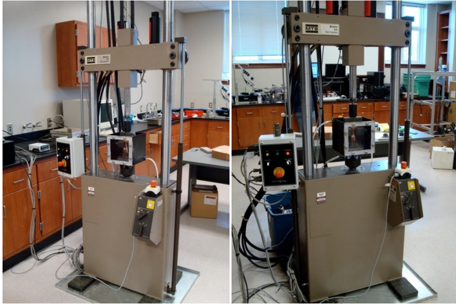
Figure 19: The MTS machine with the specialized chamber attached to the bottom of the testing plane.
